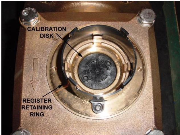
5. The calibration shaft will stay in the new position without the use of a locking device. Re-install the register and register cover assembly.
