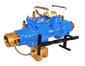
num or brass swivel and nipple, aluminum or stainless steel handles, front and rear 3" check valves, RPZ Dump Valve and adjustable support stand. The measuring element assembly includes the rotor assembly, vertical shaft and a calibration vane which eliminates the need for calibration change gears.
