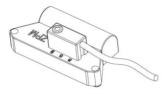
**MAGNETIC PICKUP:** Magnetic pickup from the register pointer ensures reliable positive readings.
