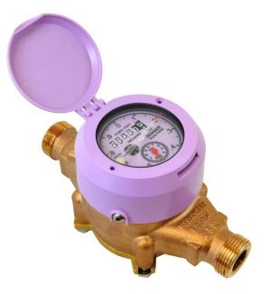
**CONSTRUCTION:** ZENNER PMNR Reclaimed Water Meters consist of three basic components: main case, measuring chamber and sealed register. The main cases are constructed using either C89833 or C89850 Brass Alloys. Measuring Chambers are constructed of a durable synthetic polymer. Registers are available as either direct read or electronic output.
