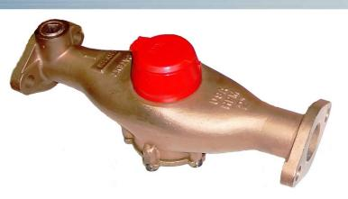
**INTRODUCTION:** ZENNER PERFORMANCE Residential Fire Meters utilize a unique patented multi-jet and dual element strainer to measure low flow rates comparable to traditional positive displacement meters with the high flows required of residential fire service meters. They are designed to measure cold and hot potable water where flow is in one direction only in residential and domestic use applications.
