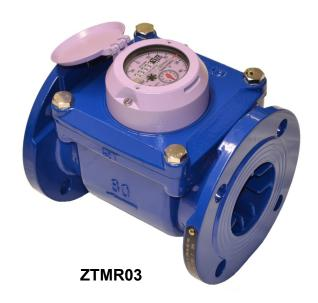
**CONSTRUCTION:** ZENNER Reclaimed Cast Iron Turbine Meters consist of four basic components: The main housing, cover plate, measuring element, and sealed register. The main housing and cover plate are made of epoxy coated ductile cast iron with round flanges, except for the 2" ZTMLR02 meter which has oval flanges. The measuring element assembly includes the rotor assembly, vertical shaft and a calibration vane which eliminates the need for calibration change gears.
