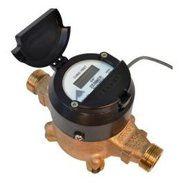
magnet located within the hermetically sealed electronic register. The gearless electronic register translates the piston oscillations into volume totalization which is both displayed on the 9 digit LCD and stored internally on a solid state microprocessor.
