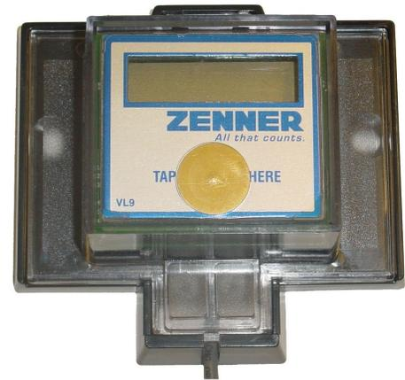
The VL-9M electronics and battery are environmentally sealed and suitable for outdoor installation, the wire terminals are not sealed for moisture. The unit should not be installed in locations below grade or in a submersible environment.
