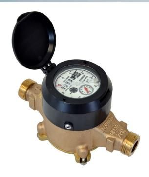
**CONSTRUCTION:** ZENNER PPD Water Meters consist of three basic components: main case, measuring chamber and a sealed register. The main cases are constructed using C89833 Brass Alloy. Measuring Chambers are constructed of a durable synthetic polymer. Bottom plates (for meter sizes 5/8" thru 1") are available in Bronze, Cast Iron or synthetic polymer. Registers are available as either direct read or electronic output.
